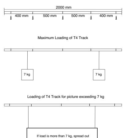
If load is more than 7 kg, spread out the load out by hanging on both corners approximately 1000 mm apart.
